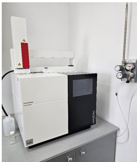
Photo 1. Device for determining sulphur at low concentrations
