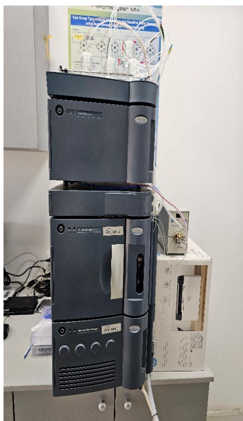
Photo 2. Equipment for the determination of polycyclic aromatic hydrocarbons in diesel derivatives
